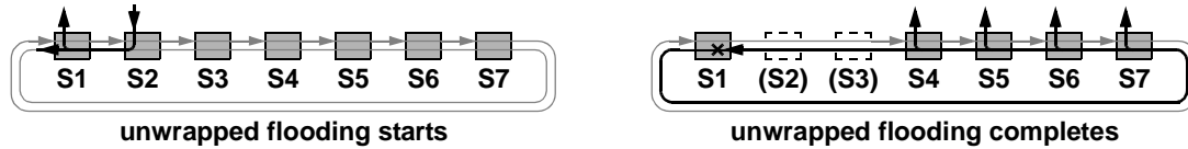
Figure A.14—Duplicate scenarios: Unidirectional source bypass
