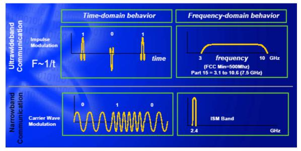
Figure 1: Impulse based waveforms compared with continuous carriers
