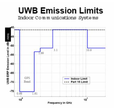
Figure 2: FCC Emission Limits for Indoor Communication systems
