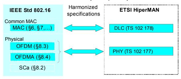
FIGURE 1 BWA Standards harmonized for interoperability for frequencies below 6 GHz
