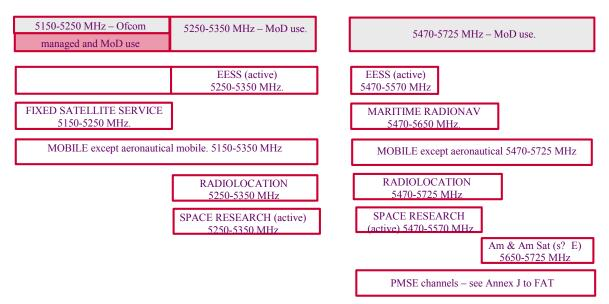
3.30 The bandplan for 5.xGHz bands A and B is shown below.
