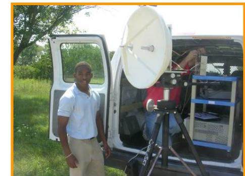
In August 2007, Battelle completed a field test to demonstrate 10 GB/s data transmission at 94 GHz.
