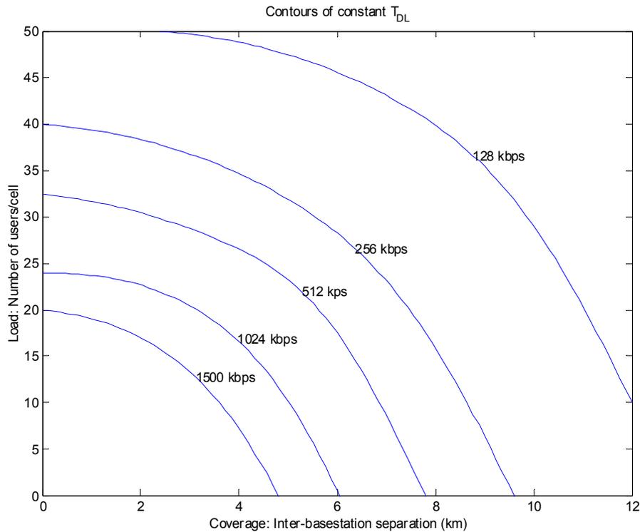
Figure 2: Contours of constant minimum service level
