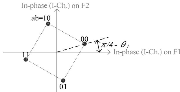
Figure 5: Signal Constellation at Transmitter Side.
