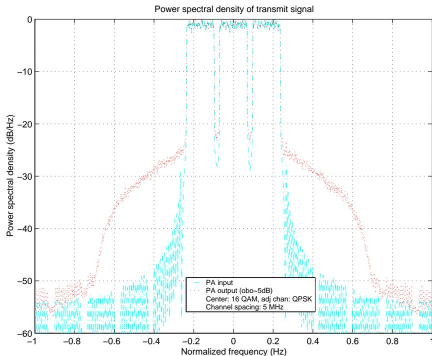
**Figure 3** Power spectral density of transmitted signal with three adjacent OFDM channels (each with 512 FFT size) with spacing at 5 MHz
