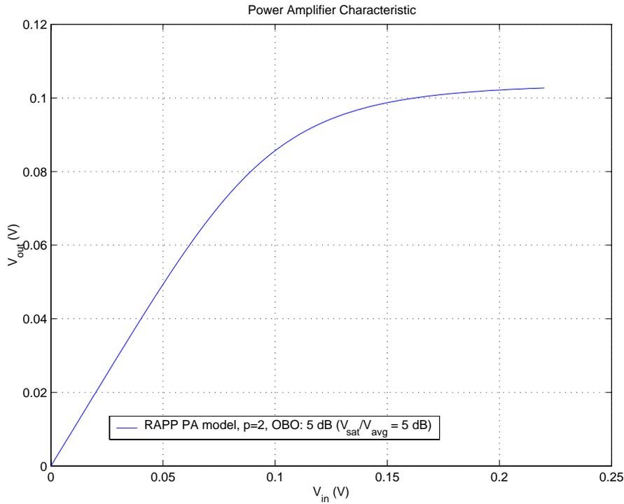
**Figure 1 AM/AM characteristics of the RAPP PA model,  $p=2$**
