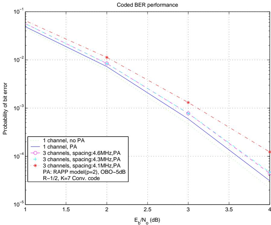
Figure 5 BER performance for various values of channel spacing, with QPSK modulation
