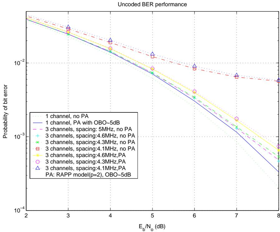
Figure 4 Uncoded BER performance for various values of channel spacing, with QPSK modulation.
