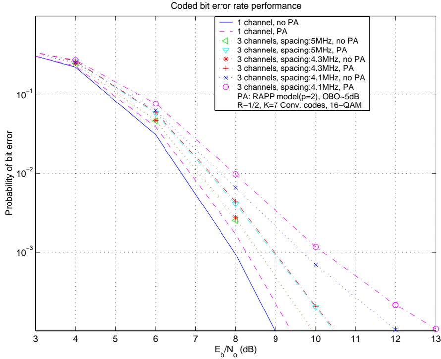
**Figure 6** Coded BER performance for case of 16-QAM, for various values of channel spacing
