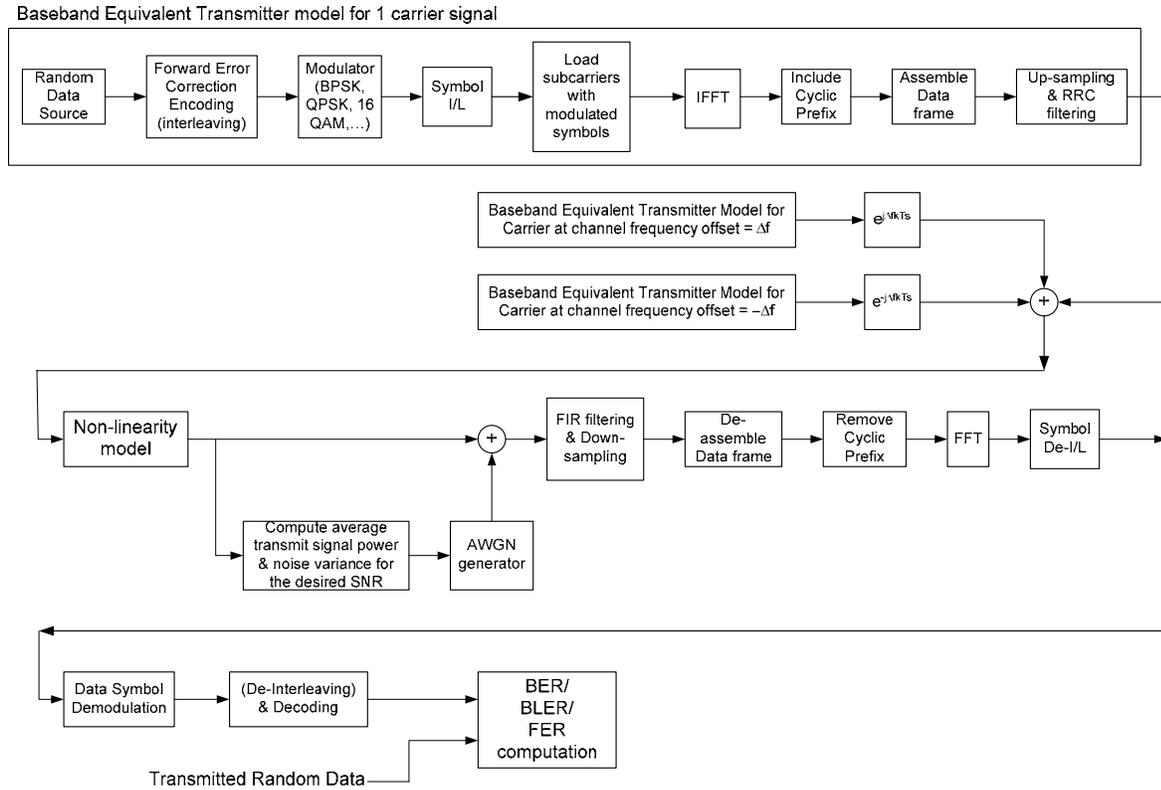
**Figure 2 Block Diagram of the simulation model**
