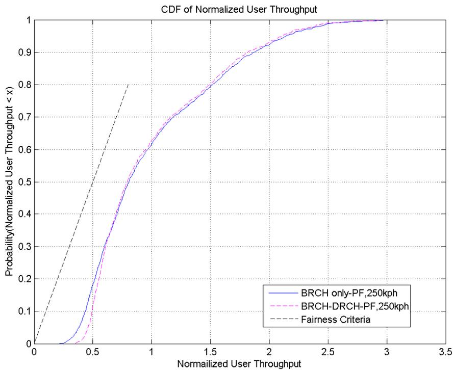
Figure 5 Normalized user throughput at 250 km/h – Fairness criteria is met
