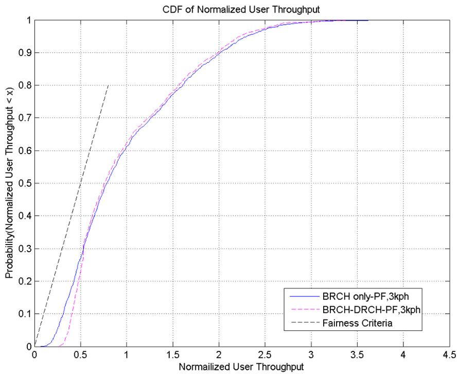
Figure 3 Normalized user throughput at 3 km/h – Fairness criteria is met
