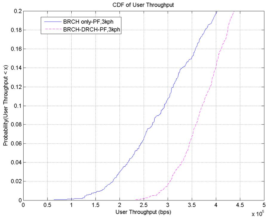
Figure 2 CDF of user throughput at 3 km/h – magnified to show cell edge performance
