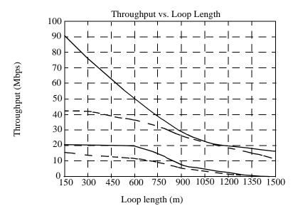
Figure 62C–3—Simulated performance of a VDSL system (using ITU-T Bandplan A) in the presence of 12 disturbers using the example PSD of this subclause and 12 disturbers using T1.417 mask SM9.
