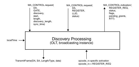
Figure 64–15—Discovery Processing Service Interfaces (OLT, broadcasting instance)
