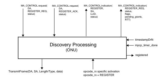
Figure 64–17—Discovery Processing Service Interfaces (ONU)
