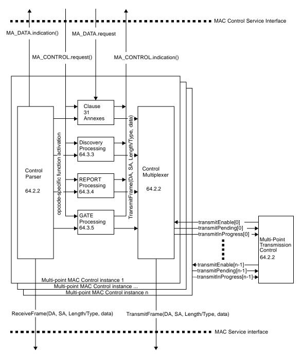
Figure 64–3—Multi-point MAC Control Functional Block Diagram
