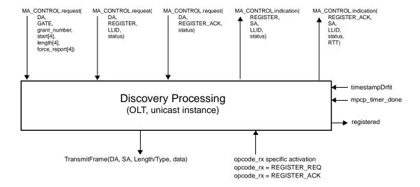
Figure 64–16—Discovery Processing Service Interfaces (OLT, unicasting instance)
