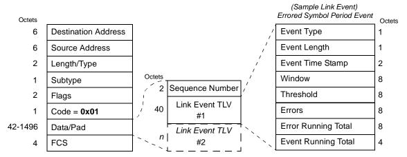
Figure 57–11—Event Notification OAMPDU frame structure
