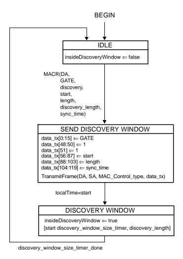
Figure 64–18—Discovery Processing OLT Window Setup State Diagram
