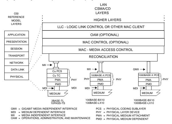
Figure 56-1—Architectural positioning of EFM: P2P Topologies
