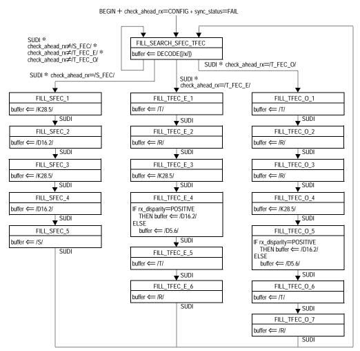
Figure 65-13—Receive buffer-fill state diagram
