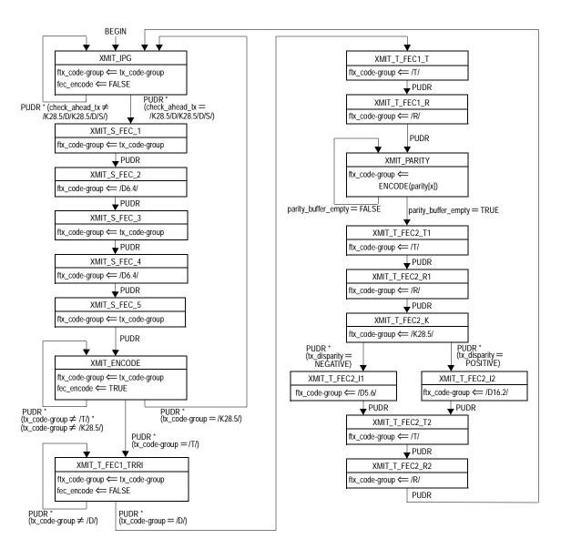
Figure 65-11—Transmit state diagram
