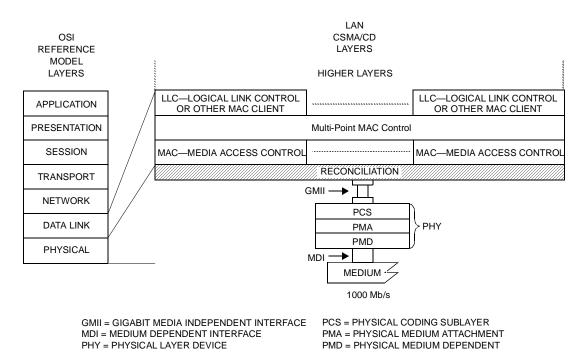
Figure 65-1—RS location in the OSI protocol stack
