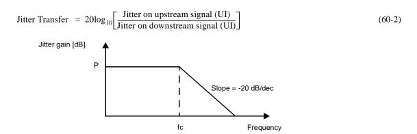
Figure 60-5—Jitter gain curve values for 1000BASE-PX10-U and 1000BASE-PX20-U
