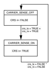
Figure 61-6—Carrier Sense state diagram
