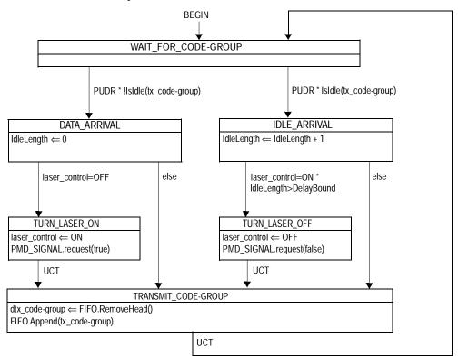
Figure 65–6—ONU data decoder state diagram
