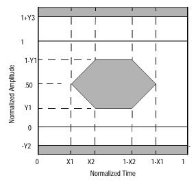
Figure 60-6—Transmitter eye mask definition
