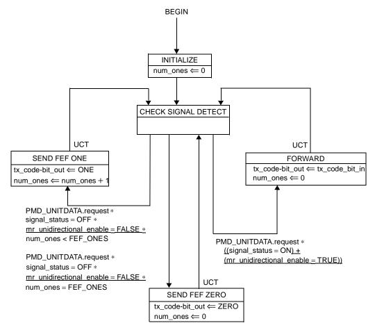
Figure 66-2—Far-End Fault Generate state diagram
