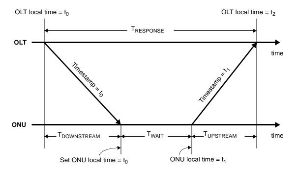
T<sub>DOWNSTREAM</sub> = downstream propagation delay
