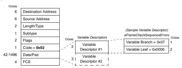
Figure 57-12—Variable Request OAMPDU frame structure
