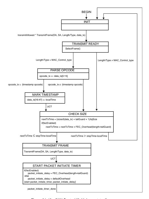
Figure 64–13—ONU Control Multiplexer state diagram
