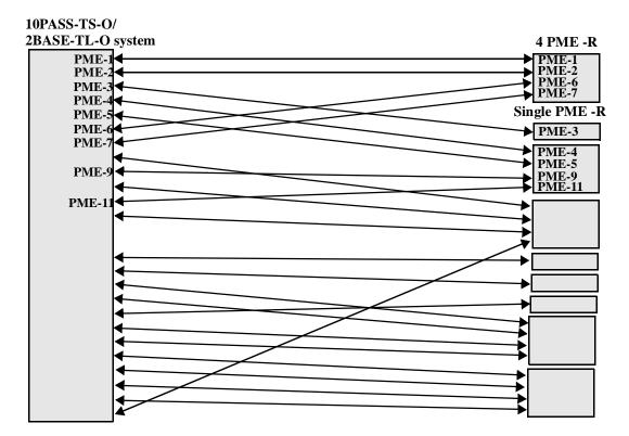
Figure 61A-2—System connectivity for discovery example
