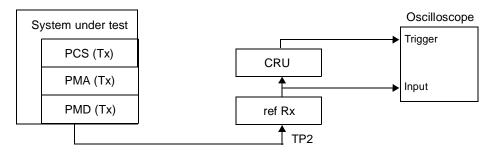
Figure 58-6—Transmitter optical waveform test block diagram
