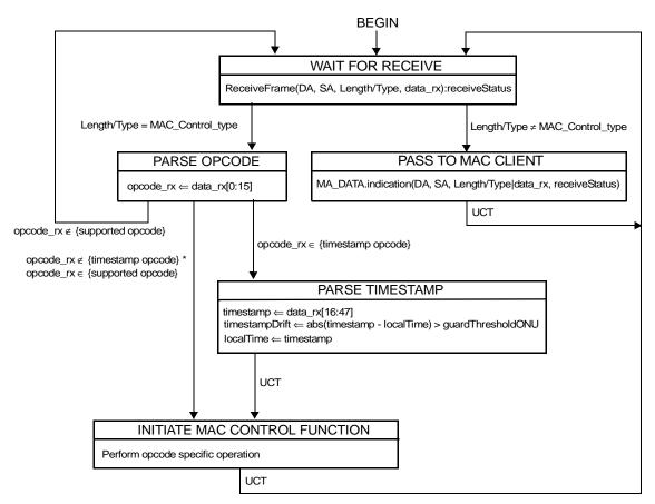
NOTE—The opcode-specific operation is launched as a parallel process by the MAC Control sublayer, and not as a synchronous function. Progress of the generic MAC Control Receive state machine (as shown in this figure) is not implicitly impeded by the launching of the opcode specific function.
