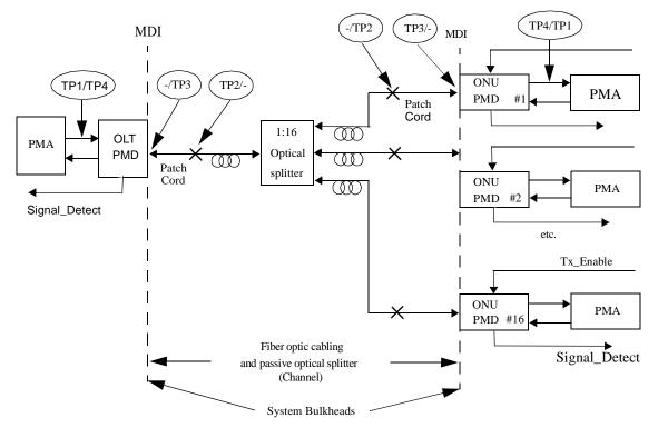
Figure 60-2-1000BASE-PX block diagram
