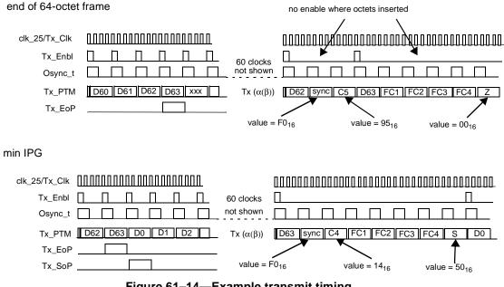
Figure 61–14—Example transmit timing
