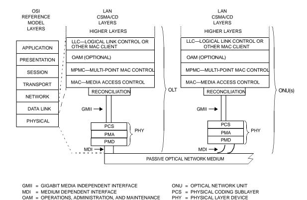
Figure 56-2—Architectural positioning of EFM: P2MP Topologies
