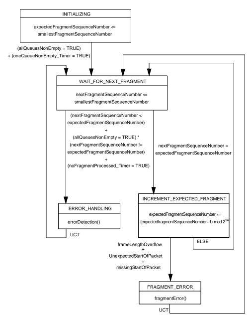
Figure 61-11—Aggregation receive function.
