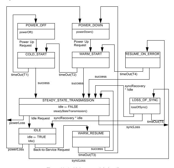
Figure 62-4—Link state and timing diagram
