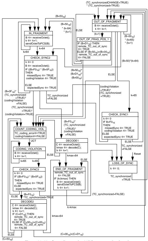
Figure 61–19—State diagram for 64/65-octet receive function
