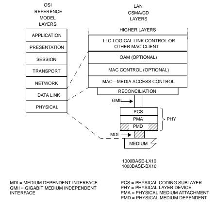
Figure 59–1—1000BASE-LX10 and 1000BASE-BX10 PMDs relationship to the ISO/IEC Open Systems Interconnection (OSI) reference model and the IEEE 802.3 CSMA/CD LAN model
