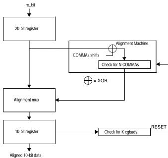
Figure 65–9—Receive synchronization block diagram
