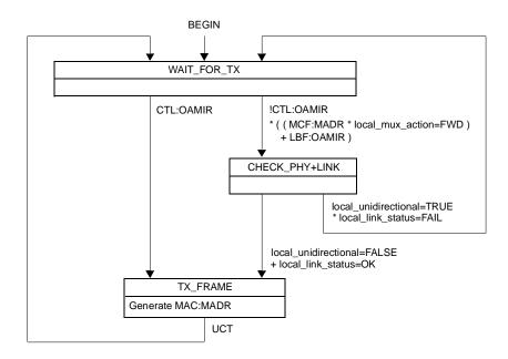
Figure 57-7—Multiplexer state diagram
