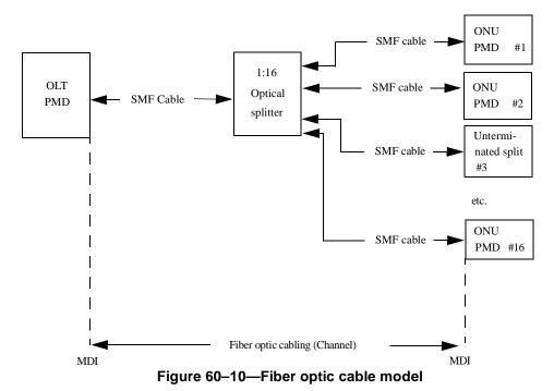
NOTE—The 1:16 optical splitter may be replaced by a number of smaller 1:n splitters such that a different topology may be implemented while preserving the link characteristics and power budget as defined in Table 60–9.
