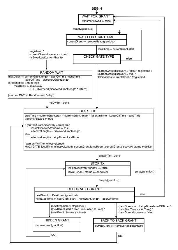
Figure 64-29—Gate Processing ONU Activation State Diagram
