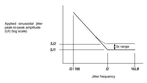
Figure 58-10—Mask of the sinusoidal component of jitter tolerance (informative)
