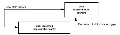
Figure 59-5—Utilization of clock recovery unit during measurement
