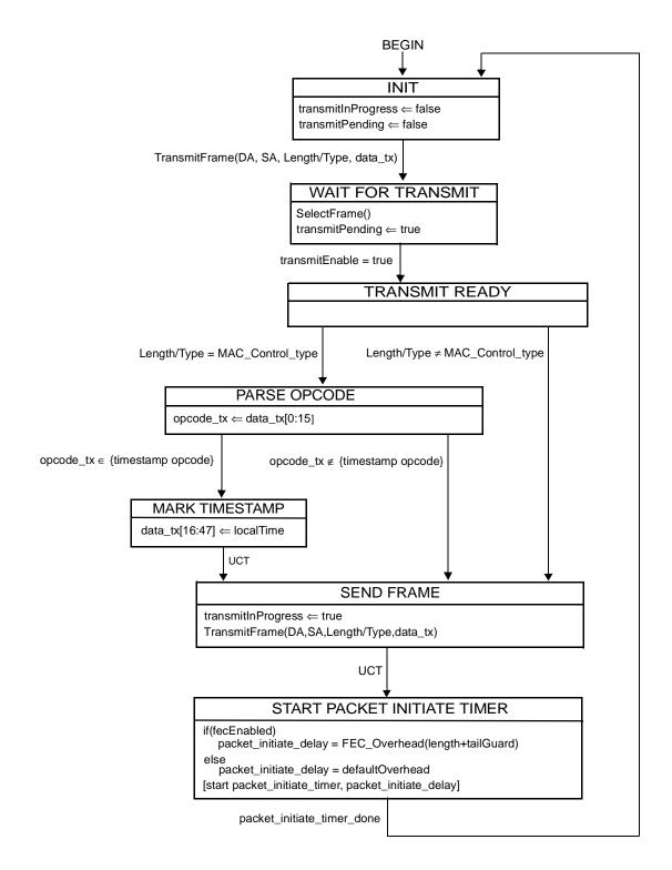
Figure 64-12-OLT Control Multiplexer state diagram
