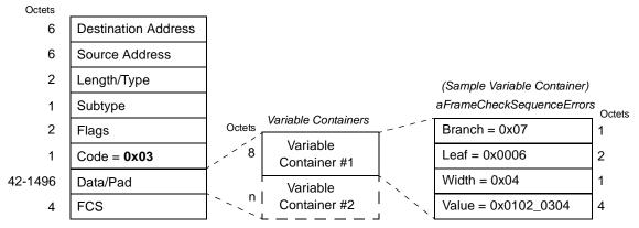
Figure 57–13—Variable Response OAMPDU frame structure
