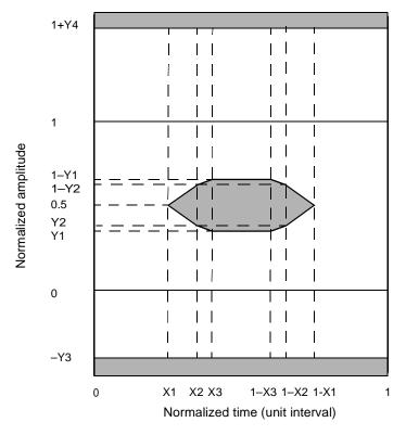
Figure 58–5—Transmitter eye mask definition
