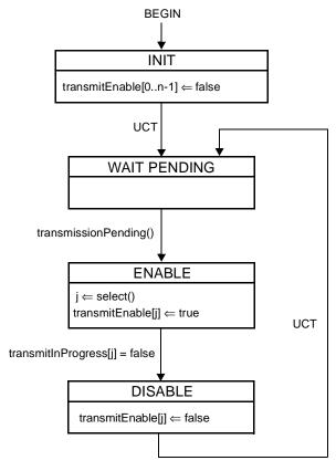
Figure 64–9—OLT Multi-Point Transmission Control state diagram
