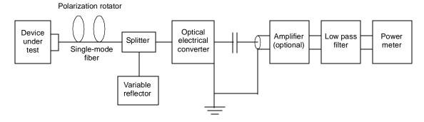
Figure 58-4—RIN<sub>x</sub>OMA measurement setup
