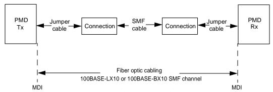
Figure 58–12—Fiber optic cabling model
