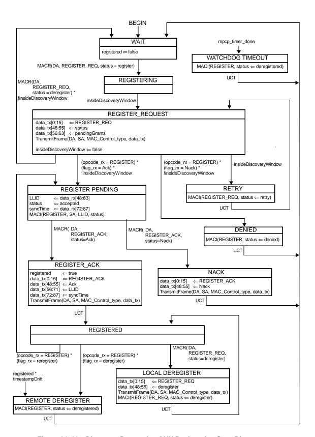
Figure 64–22—Discovery Processing ONU Registration State Diagram
