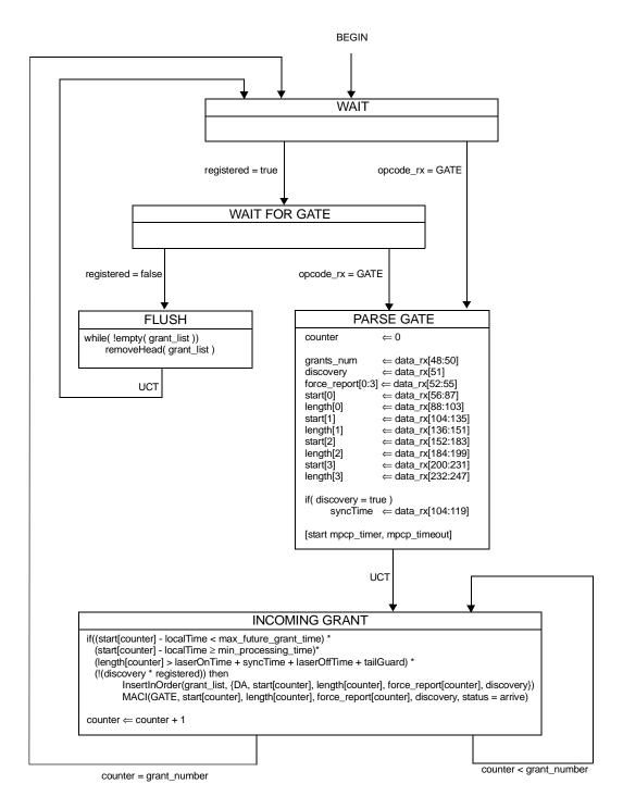
Figure 64-28—Gate Processing ONU Programing State Diagram
