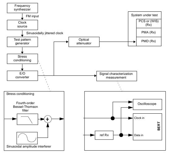
Figure 58–8—Stressed receiver conformance test block diagram
