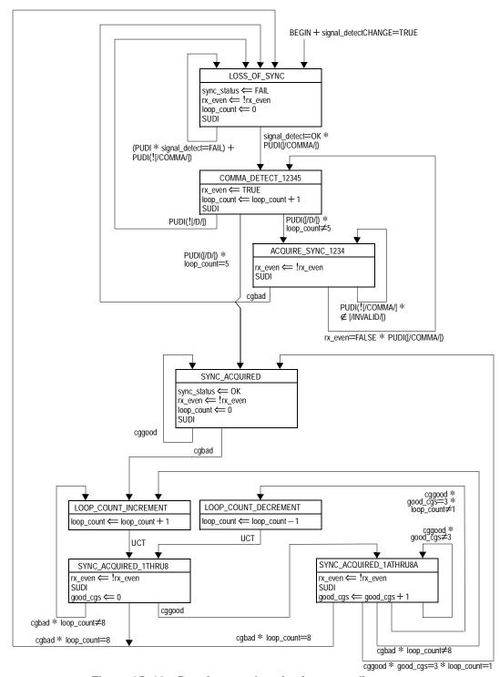
Figure 65-12—Receive synchronization state diagram
