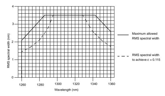
Figure 60-3—1000BASE-PX10-U transmitter spectral limits
