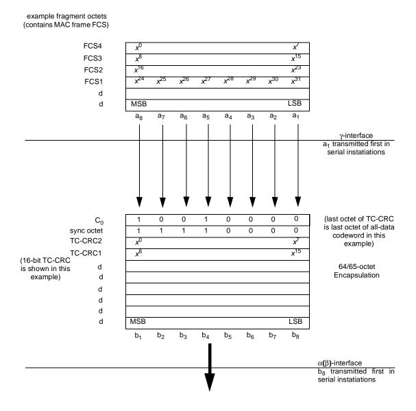
Figure 61–16— $\gamma$ -interface to  $\alpha(\beta)$ -interface bit ordering
