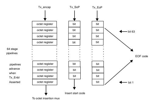
Figure 61-13—Example transmit pipeline
