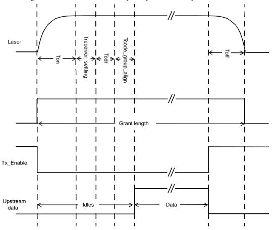
Figure 60-7—P2MP timing parameter definition
