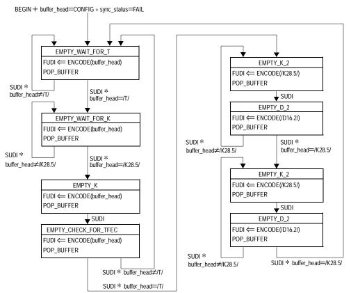
Figure 65-14—Receive buffer-empty state diagram
