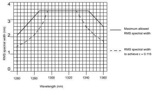
Figure 59-3—1000BASE-LX-10 Transmitter spectral limits
