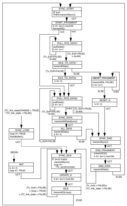
Figure 61–18—State diagram for 64/65-octet transmit function
