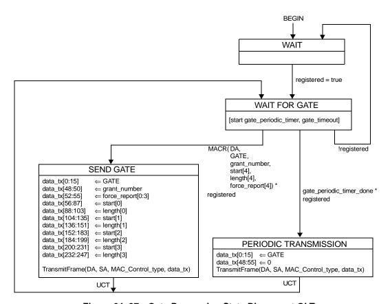
Figure 64–27—Gate Processing State Diagram at OLT
