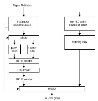
Figure 65-10—Receive data block diagram
