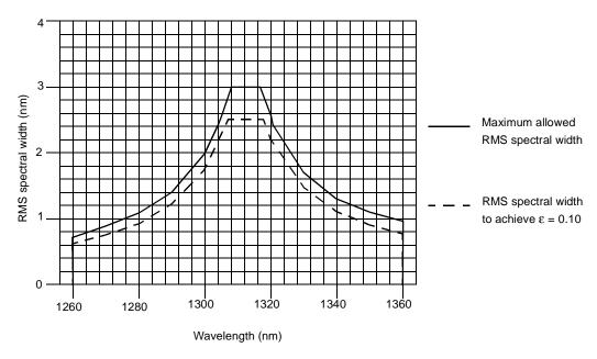
Figure 60-4—1000BASE-PX20-U transmitter spectral limits
