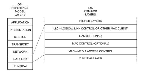
Figure 57–1—OAM sublayer relationship to the ISO/IEC Open Systems Interconnection (OSI) reference model and the IEEE 802.3 CSMA/CD LAN model
