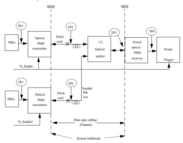
Figure 60–9—Receiver settling time measurement setup
