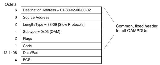
Figure 57-9—OAMPDU frame structure
