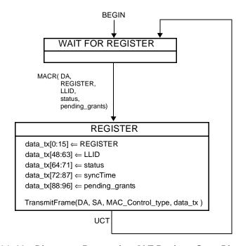
Figure 64–20—Discovery Processing OLT Register State Diagram
