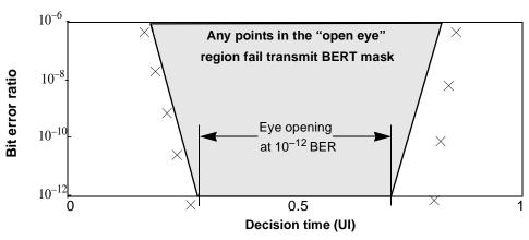
Figure 58-11—Example transmit BER mask at TP3
