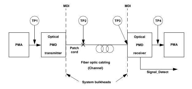
Figure 58-2—100BASE-X block diagram
