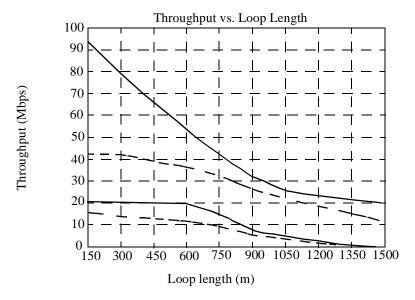
Figure 62C-2—Simulated performance of a VDSL system (using ITU-T Bandplan A) in the presence of 24 disturbers using the example PSD of this subclause.
