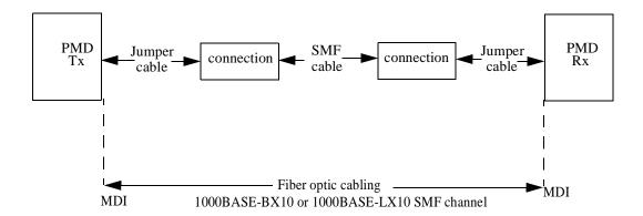
Figure 59-7—Fiber optic cable model
