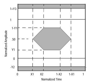
Figure 59-4—Transmitter eye mask definition
