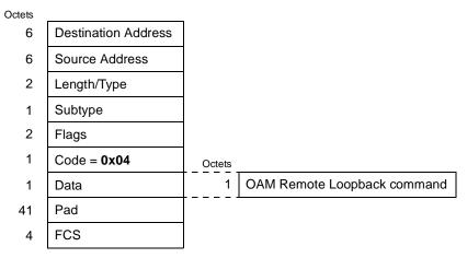
Figure 57-14—Loopback Control OAMPDU frame structure
