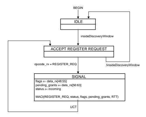
Figure 64–19—Discovery Processing OLT Process Requests State Diagram
