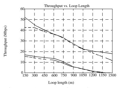
Figure 62C-4—Simulated performance of a VDSL system (using ITU-T Bandplan A) in the presence of 12 disturbers using the example PSD of this subclause and 12 disturbers using T1.417 mask SM6.
