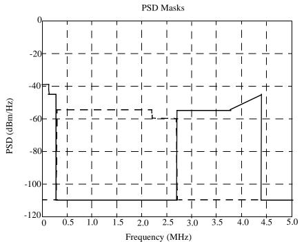
Figure 62C-1—Example PSD Masks for MCM 10PASS-TS
