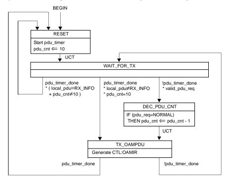
Figure 57-6—Transmit state diagram
