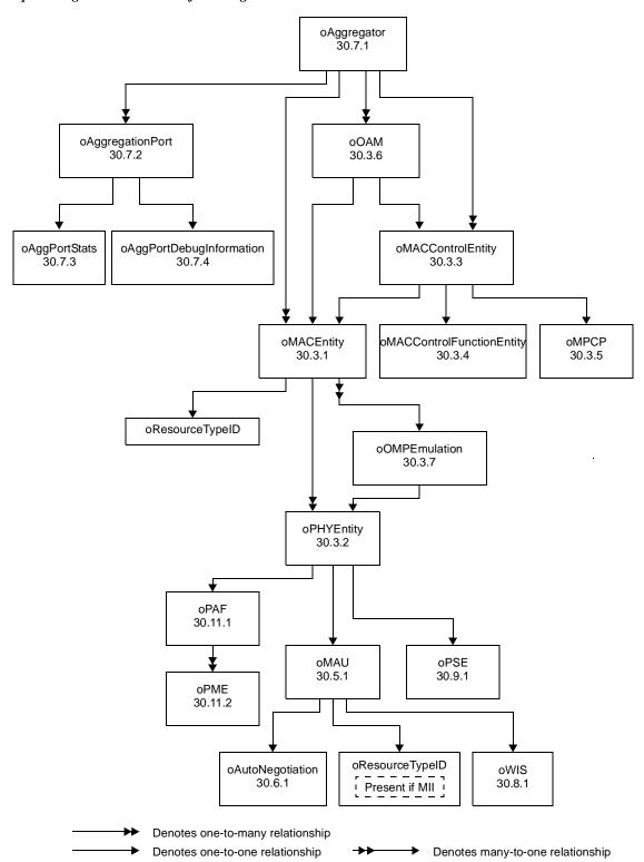
Figure 30-3—DTE System entity relationship diagram
