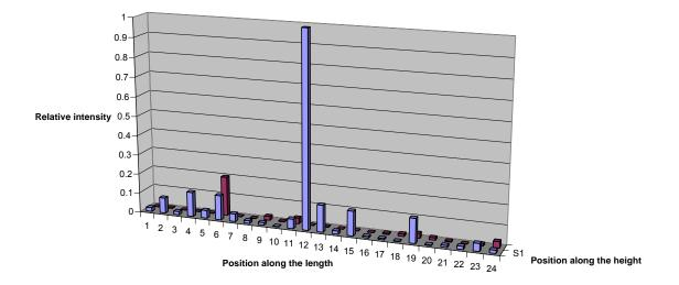
Figure 7: Relative PSAELFEXT contributions from disturber channels.
