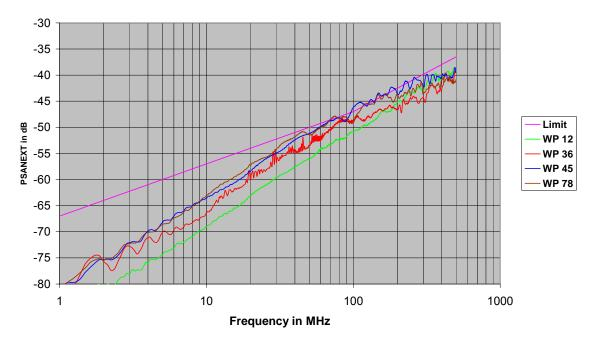
Figure 4: PSANEXT of victim channel 12 to all 47 disturber channels.
