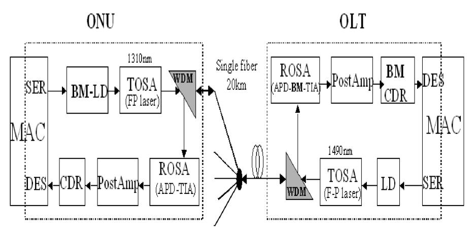
Downstream CM PX20 1490nm: Tx power +2dBm(min) to Rx sens -27dBm (max.) FP is assumed in specs but DFB is actually used for better disp. tolerance
