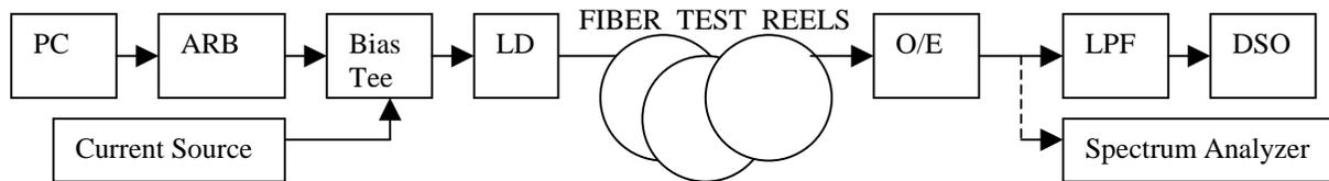
Figure 2. Experimental setup.
