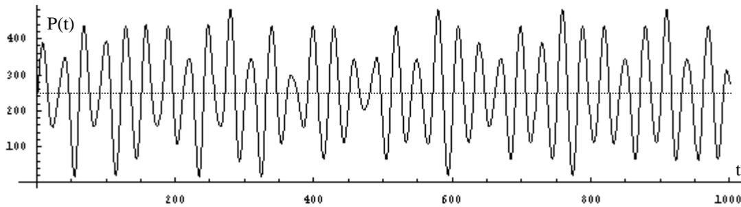
Figure 1. Output of laser diode pigtail,  $n = 10$  levels,  $m = 6$ ,  $P_{avg} = 3\text{mW}$ , 200 psec per step.
