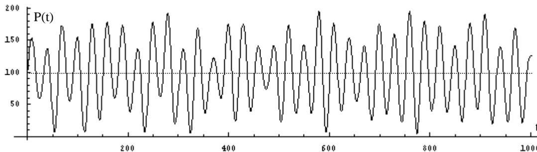
Figure 3. Received signal after 10 km of multimode fiber,  $P_{avg} = 7 \mu\text{W}$ , 200 psec per step.
