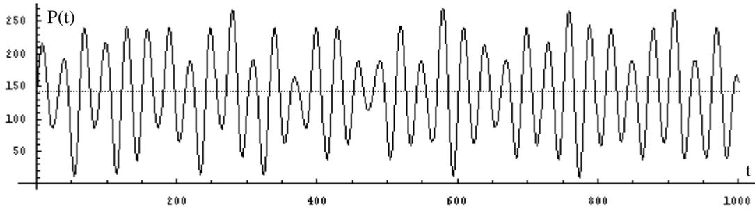
Figure 4. Received signal after 50 km of singlemode fiber,  $P_{avg} = 5 \mu\text{W}$ , 200 psec per step.
