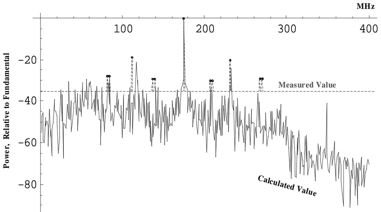
Annotated Figure. Computed spectrum of launched signal (solid line) and measured spectrum (dashed line) showing spectrum analyzer noise floor and 11 observed peaks ( $\cdot$  points).
