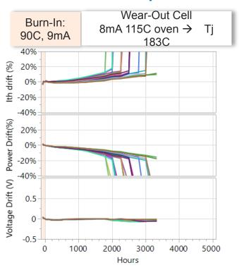
Example 850nm 22 units at similar accelerated stress conditions Wafer passes 100G requirement for 20yrs at 8mA 85°C Power & Ith observed >600hrs with catastrophic failures >1,600hrs
