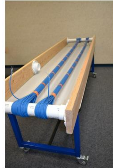
Figure C.3 - Test set-up for cable bundles in air.
