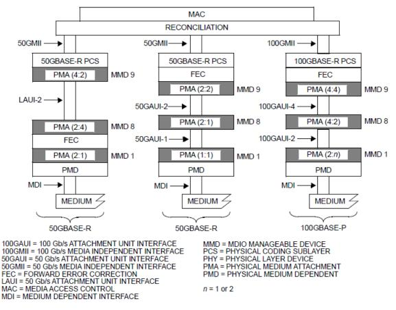
Figure 135-2—Example 50GBASE-R and 100GBASE-P PMA layering
