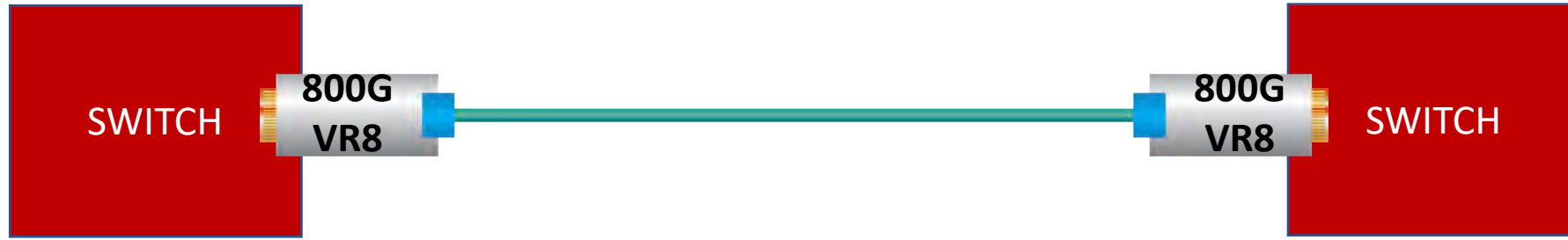
VR8 module shown in 800G point-to-point link over 50m
