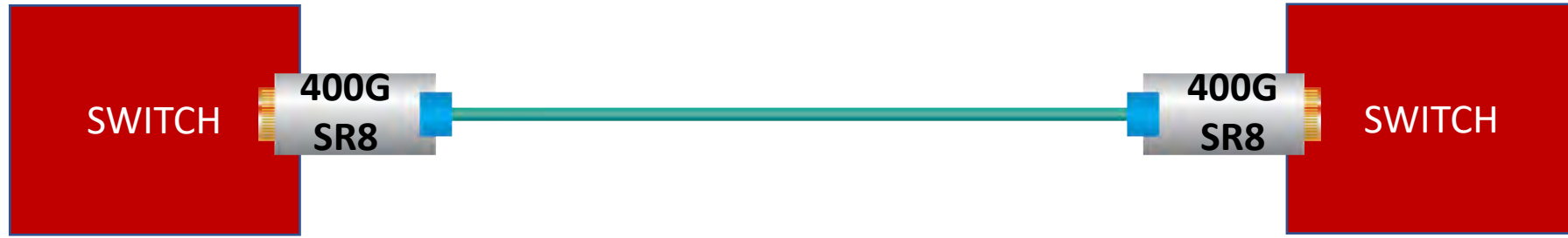
SR8 module shown in 400G point-to-point link
