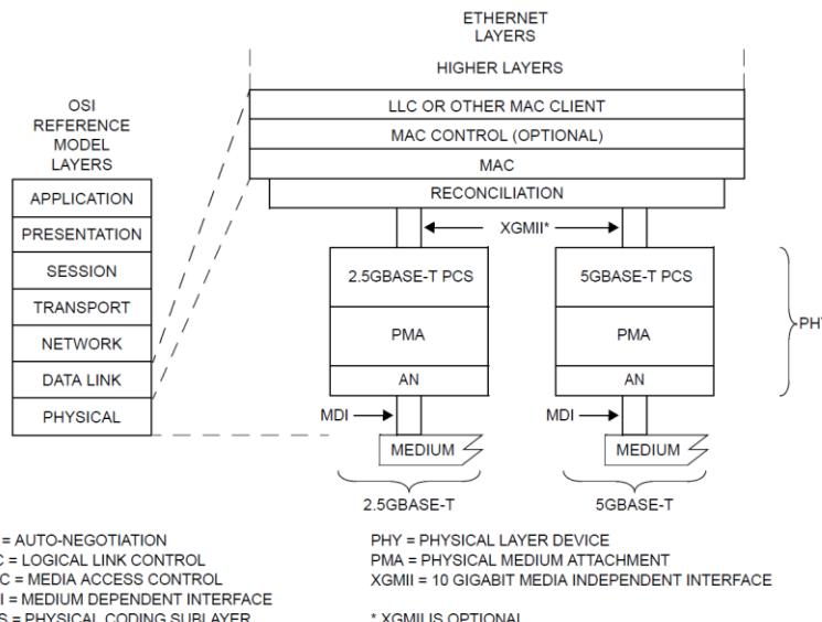
Figure 125-1—Architectural positioning of 2.5 Gigabit and 5 Gigabit Ethernet
