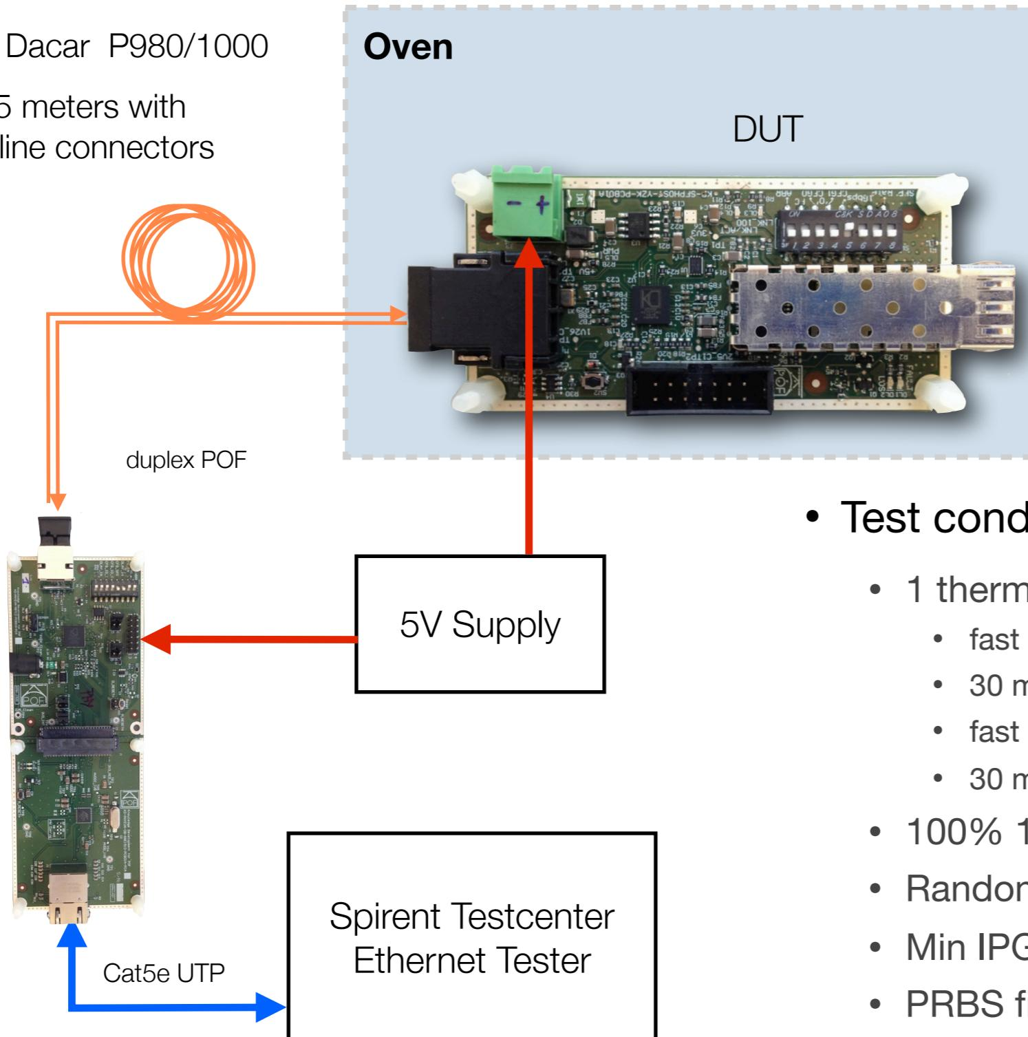
Line loopback is configured in POF PHY (received Eth frames are looped back at GMII and retransmitted to PCS TX for verification by Spirent connected to link partner)
