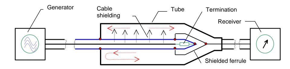
IEC 62153-4-3/-4-4 Metallic communication cable test methods, EMC EN 50289-1-6 Communication cable, Electromagnetic performance
