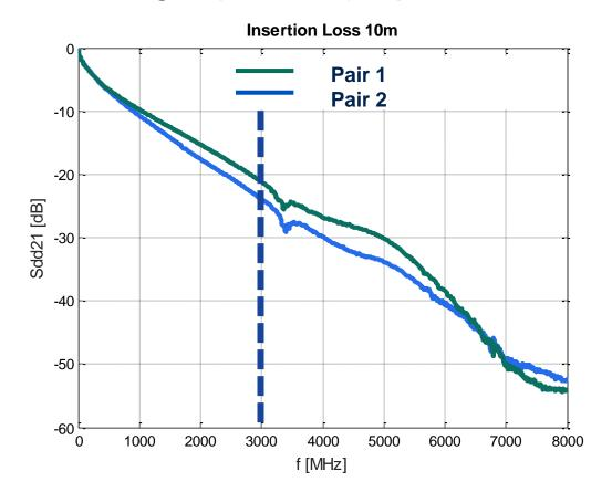
2 x 3 GHz bandwidth is realistic with good STQ cables
