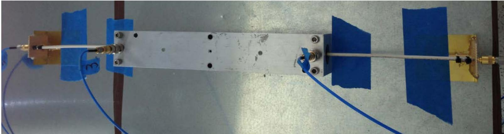
10 AWG conductor directly attached to SMA with the SMA grounded through a 5 cm (2 in) brass plate
