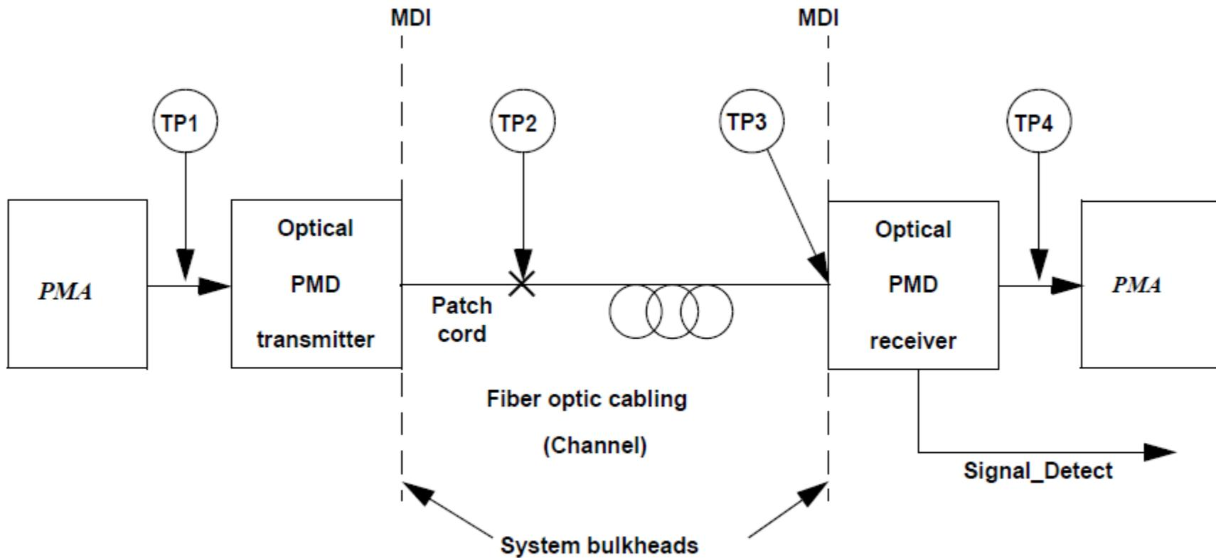
Figure 59-2—1000BASE-X block diagram
