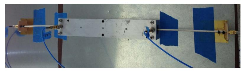
10 AWG conductor directly attached to SMA with the SMA grounded through a 5 cm (2 in) brass plate
