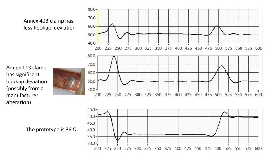
A 61 cm (24 in) reference wire is used in the clamps to compare injection levels
