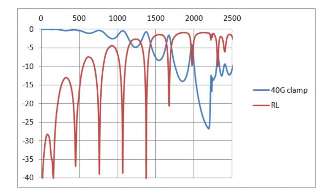
While the clamp Insertion Loss and Return Loss become extreme out at 2 GHz, clamp transmission is operational out to 2.2 GHz
