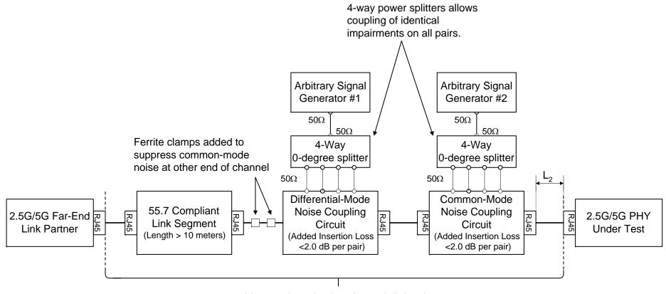
Measure insertion loss for each link pair between these points terminated by 100  $\,\Omega$
