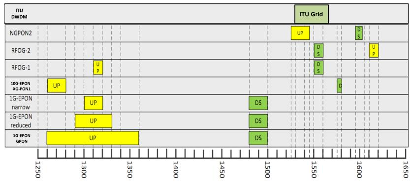
Current allocations support coexistence by providing non blocking optical BW plus adequate guard band separation
