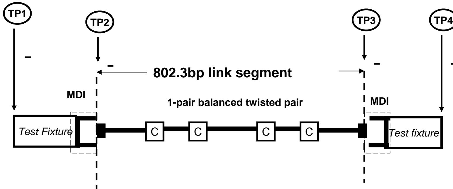
Link segment transmission and coupling parameters – TP2-TP3
