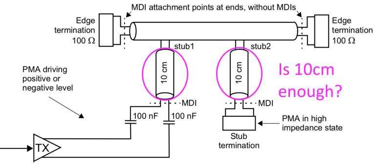
Figure 147–20—Multidrop line termination and PMA
