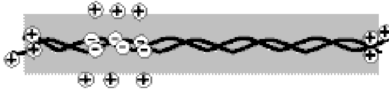
Figure 1 Tribocharging example 1. For simplicity, only one twisted pair is shown.
