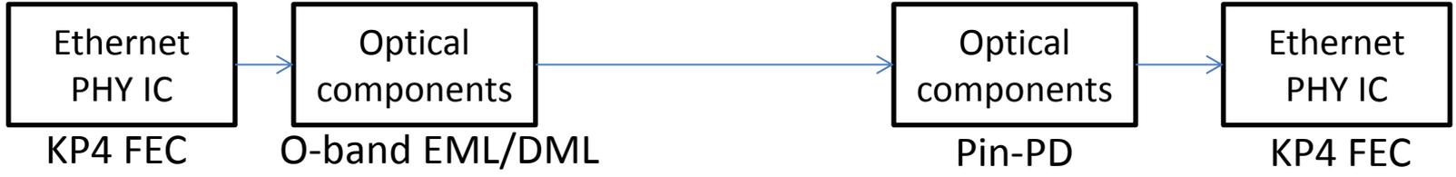
Example configurations for 40km(5x80G) Not necessary to use all the functions
