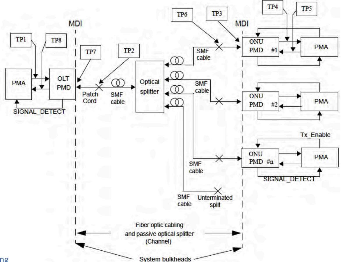
Figure 75-3—10GBASE-PR and 10/1GBASE-PRX block diagram
