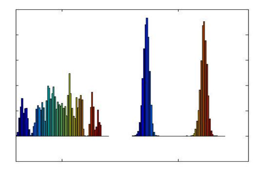
Histogram: Input to Equalizer Histogram: Equalized Signal At DFE Slicer
