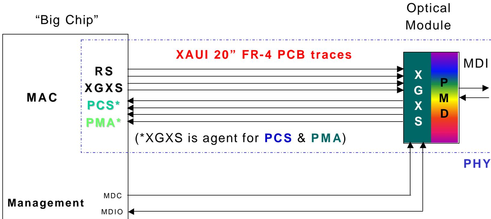
E.g. Switch port, no XGMII, integrated MAC/RS/XGXS, 20" XAUI on 2 cards + backplane Retimer/Repeater In Optical Module to attenuate jitter
