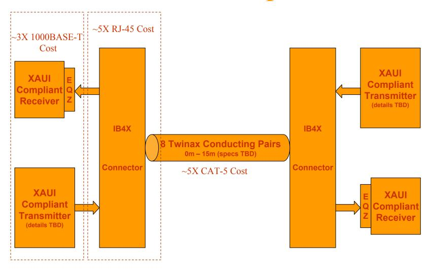
IB4X refers to the InfiniBand 4X copper physical layer specified by the InfiniBand Trade Association
