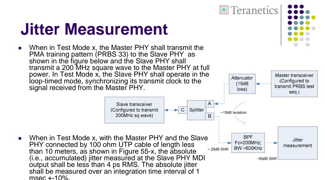
Note: 4 ps RMS jitter corresponds to an SNDR of 46 dB at 200 MHz.
