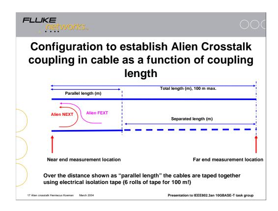
This slide shows the test configuration of the Category 6 cables with enhanced Alien Crosstalk performance to determine the properties as a function of joint by taping length. This experiment was NOT conducted on the Category 5e rated cable.
