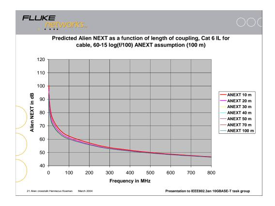
This slide shows the prediction of Alien NEXT when the length over which the coupling takes place is less than 100 m. An "average" Alien NEXT limit is used for comparison purposes.
