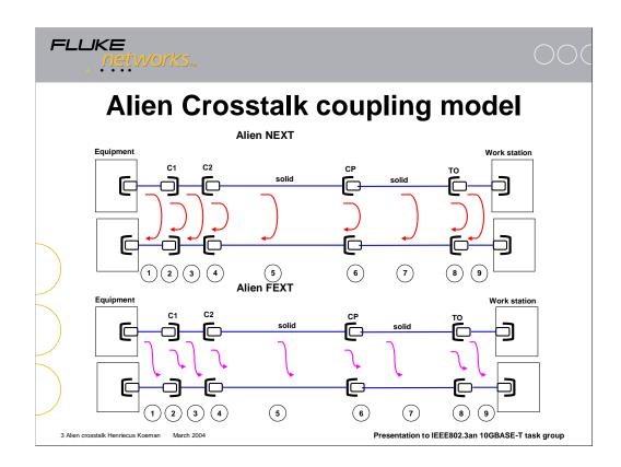
This slide shows the generic Alien NEXT and Alien FEXT models of two channels. While the diagrams show channels of equal length, that is not intended to be the case.
