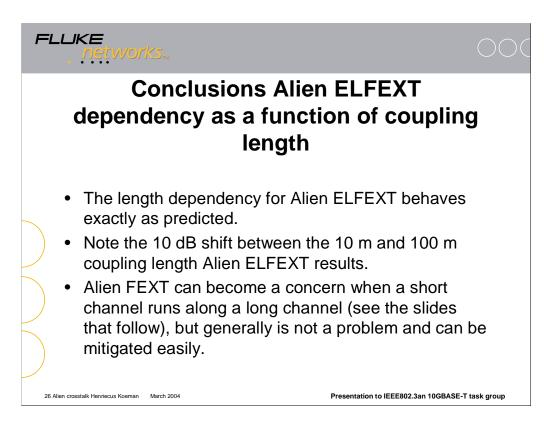
The length dependency for ELFEXT was confirmed in this experiment and can be used for channel modeling purposes.
