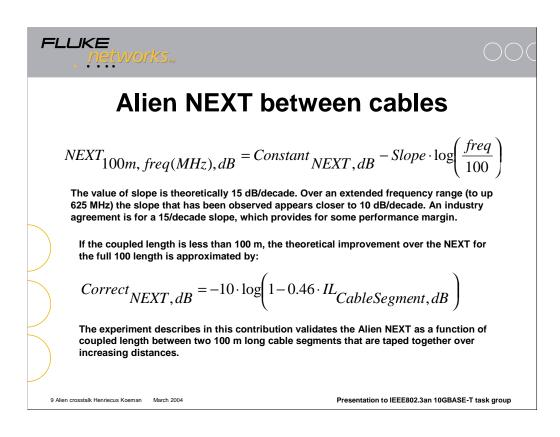
The equations shown in this slide are applicable to NEXT within a cable jacket. At first sight there is no reason to question the validity of these equations for Alien NEXT between cables. For NEXT within a cable, a 15 dB/decade slope is applicable. It is the opinion of the author, based on practical measurements, that the Alien NEXT is better approximated with a 10 dB/decade slope. Generally assumed is the 15 dB/decade slope, which provides for some performance margin.
