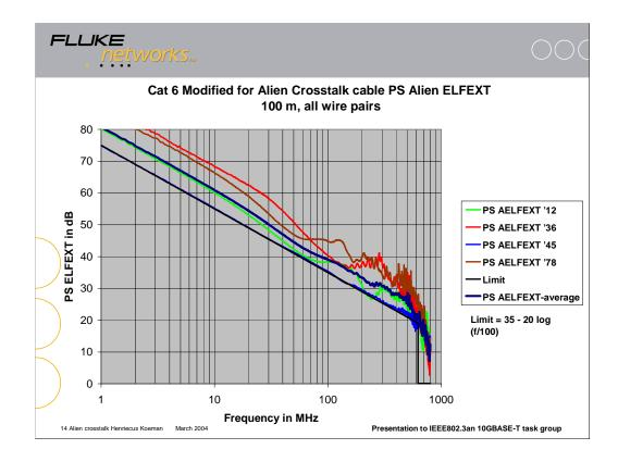
This slide shows the measured Alien ELFEXT results for the category 6 cable with enhanced Alien Crosstalk performance. This measurement took place when two cables were taped together over the full 100 m length.
