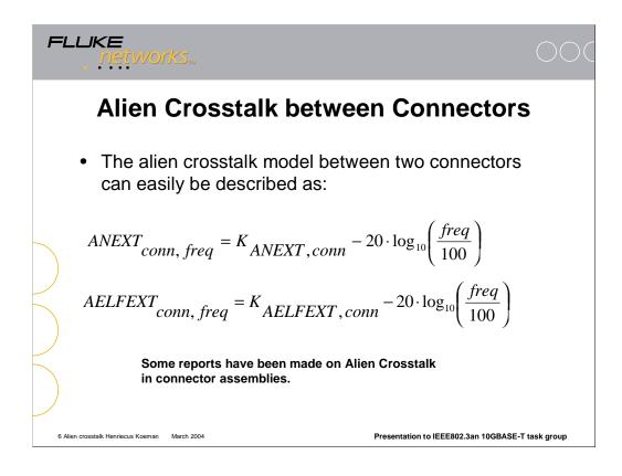
It may be expected that the Alien Crosstalk between connectors (of a patch panel or multiple telecommunications outlets or the connectors of a consolidation point) is well behaved and will show a dependency as a function of frequency that has a 20 dB/decade slope.
