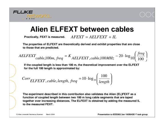
As far as Alien ELFEXT is concerned: a model is adopted that matches the ELFEXT within a cable. It is shown that predictions are that the frequency response is exhibits a 20 dB/decade slope. The response is smooth, unlike NEXT. The only deviation from the predicted slope originates from delay skew and a very few nulls may be present in the response towards the high frequency end.
