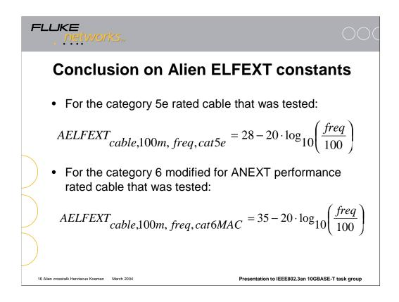
Conclusions were that the cables that were tested had the properties as shown in this slide. These results can be used for modeling purposes, predictions of the boundary of channel Alien Crosstalk performance.
