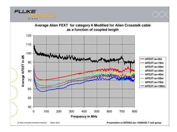
This slide shows the actually measured FEXT data (rather than ELFEXT data which has the insertion loss subtracted).
