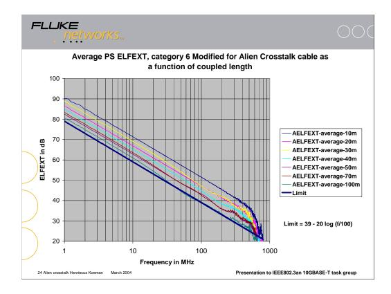
The ELFEXT result which was computed from the FEXT and insertion loss results is shown in this slides. It is obvious that the slope remains 20 dB/decade.
