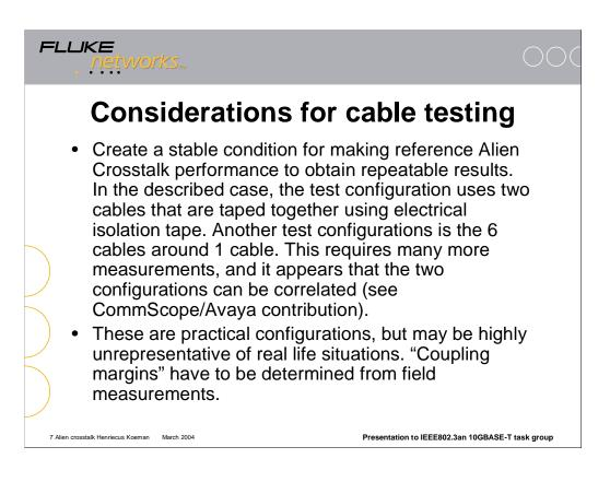
For reference measurement purposes, it is essential to create test conditions that provide for consistent test results. In particular, it appears insufficient to use cable ties that do not ensure that the jacket of the cable is touching over the full length of the cable that is tested. It is easily shown that small air gaps will enhance the measured results significantly.
