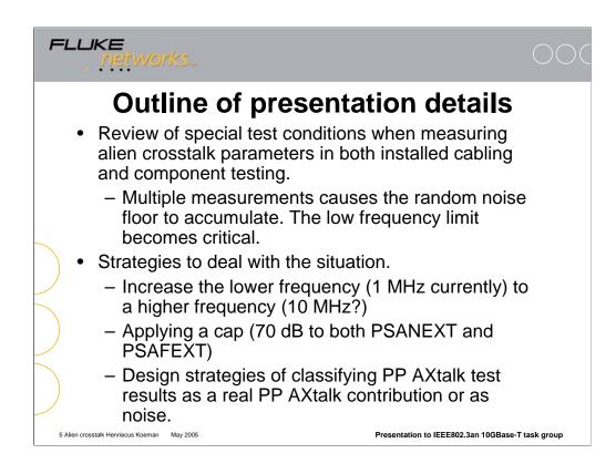
The detailed aspects of this presentation discuss the special test conditions when measuring alien crosstalk parameters in both installed cabling and component testing.
