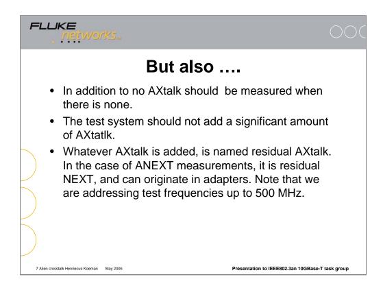
Of course, one should not measure any Alien Crosstalk, if there is nothing connected to the test system. The residual Alien NEXT is measured by further extending the averaging and measurement times to reduce the influence of random noise. Practically, there is a limit of what additional averaging really does, though. So some influence of random noise on the measured result remains visible.
