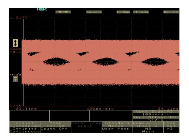
• Eye diagram of a PRBS-31 data pattern after the data path
