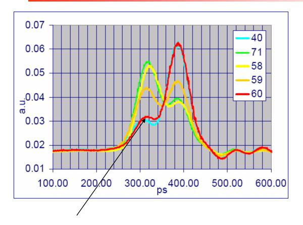
Corning experience is that we don't see the "infinite bandwidth" with 0um-1um launch with fibers with pulse splitting which is noticeable with 4um offset.
