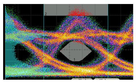
Histogram over 1 UI (same as asynchronous measurement)
