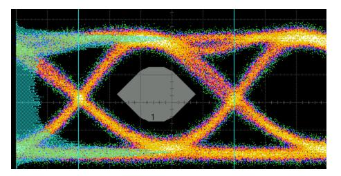
Histogram over 1 UI (same as asynchronous measurement)
