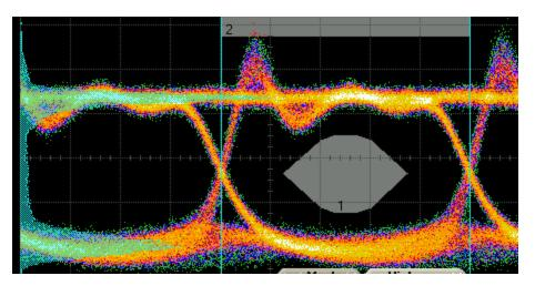
Histogram over 1 UI (same as asynchronous measurement)
