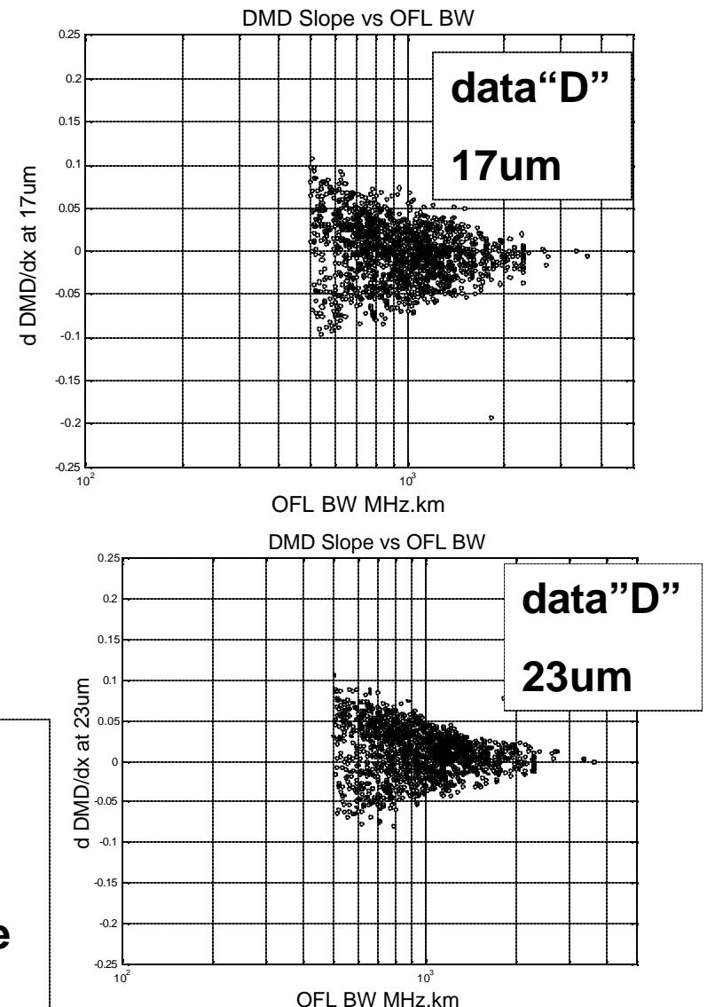
**The advantage of plotting DMDslope vs. OFL BW is that this information is available in the historical production data sets “B” and “D”.**
