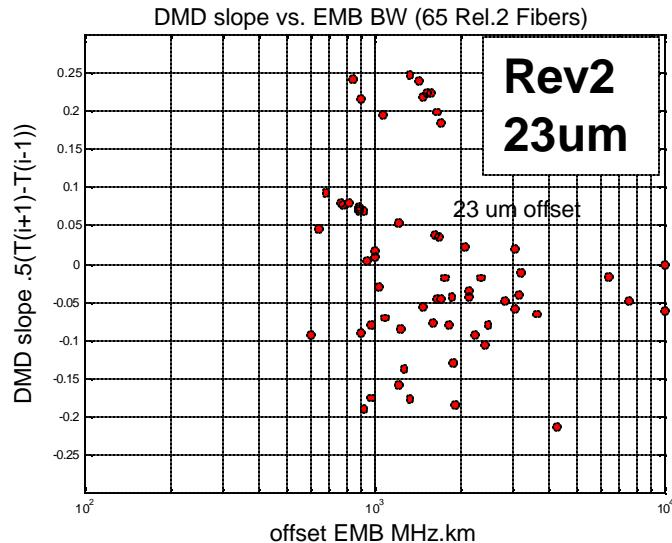
**Slope vs. EMB has “V-shaped” structure along with outliers inside the “V”. Points with offset EMB>2000MHz. km are no-problem for this launch.**
