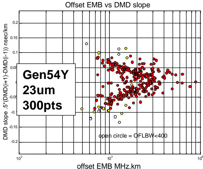
**The Gen54 mode delays retrain the V-structure but show lower peak BWs than the MBI310, consistent with the pre-GbE DMD & OFL BW data**
