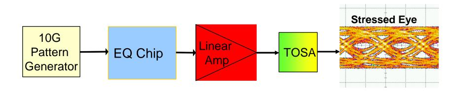
The Stressed Eye Generator can be programmed to emulate LRM TP3 Test by programming taps of the EQ chip
