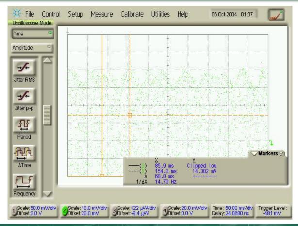
RX Time-domain signal. Expanded time-base. 7Hz, 1G acceleration (5mm deflection). Higher harmonic channel variations much smaller in magnitude as indicated in spectral analysis, Eg 21Hz.
