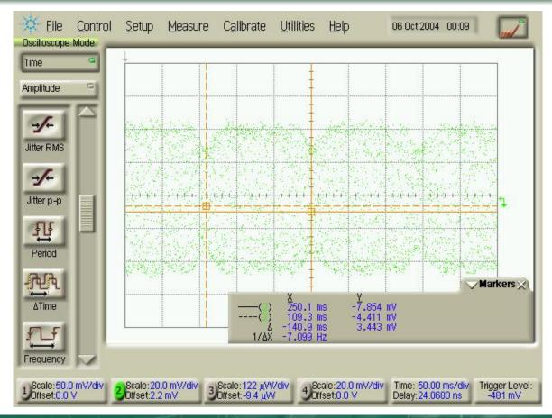
RX Time-domain signal. Expanded time-base. 7Hz, 1G acceleration (5mm deflection). Higher harmonic channel variations much smaller in magnitude as indicated in spectral analysis, Eg 14Hz.
