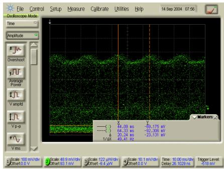
20 Hz vibration frequency, 20 Hz channel variation
