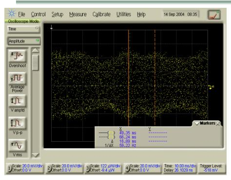
Channel variations at harmonics of the mechanical vibration frequency are visible in the time domain.
