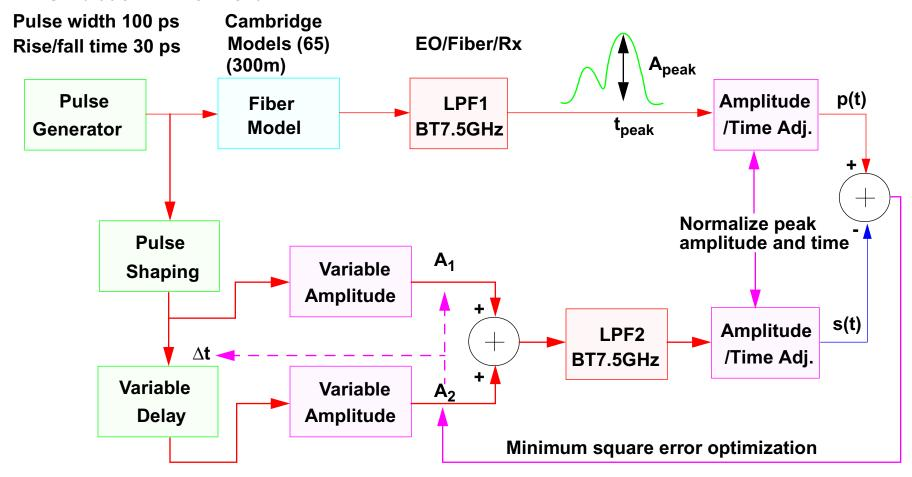
The simulation environment for fiber path consists of the fiber model (Cambridge model), a BT LPF 7.5 GHz and a normalization block to adjust for peak amplitude value and time.
