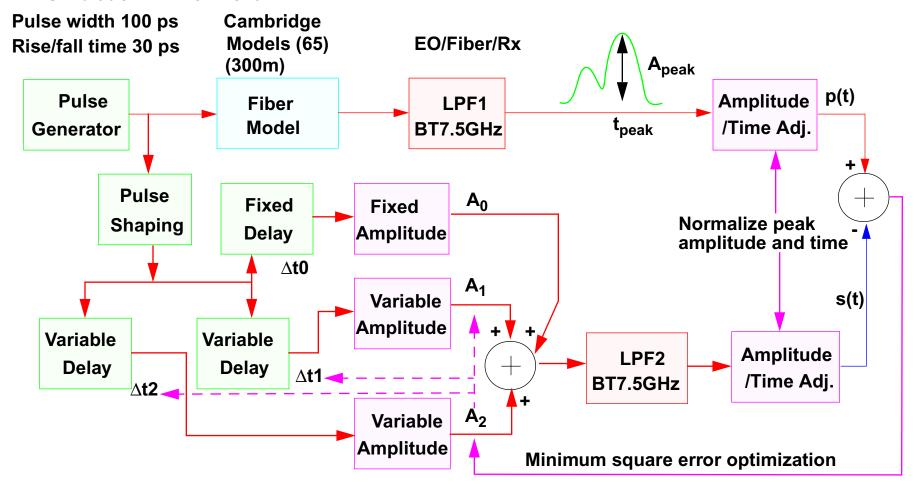
There are three delay blocks in the simulation environment. We can adjust  $\Delta t1$  and  $\Delta t2$  relative to  $\Delta t0$  such that the two peaks can be symmetrical relative to the main pulse  $A_0$ , or on the same side (precursor or post-cursor).
