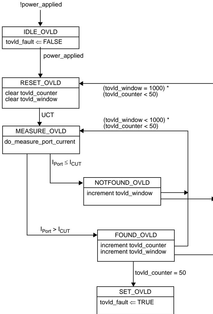
Figure 33–1—PSE monitor overload state diagram
