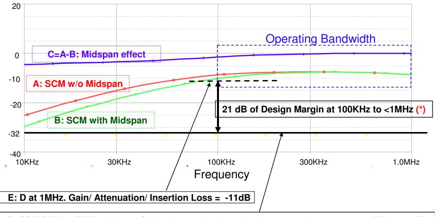
D: SCM PHY to PHY minimum Gain/ Attenuation/ Insertion Loss requirements at 100MHz= -32dB
