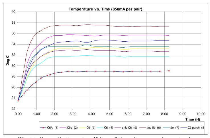
When tested in an ambient temperature ~23 degrees C, the maximum measured temperature rise was 15 degrees C for a current level of 850 mA per pair. Although the higher categories of cabling faired better (Maximum temperature rise for C6A was measured at 6 degrees C), overall, this level of current exceeded the guidance of 10 deg C maximum temperature rise for performance and longevity.
