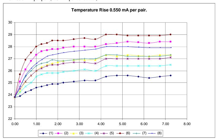
With a maximum current of 550 mA per pair, the maximum measured temperature rise was less than 7 degrees on all categories of cabling. This temperature rise is acceptable both in terms of its effect on performance and its effect on longevity.
