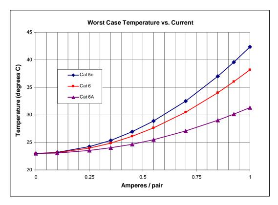
Cabling standards specify the IL loss de-rating at 0.4% per degree C. The effect of temperature rise on IL is being studied.
