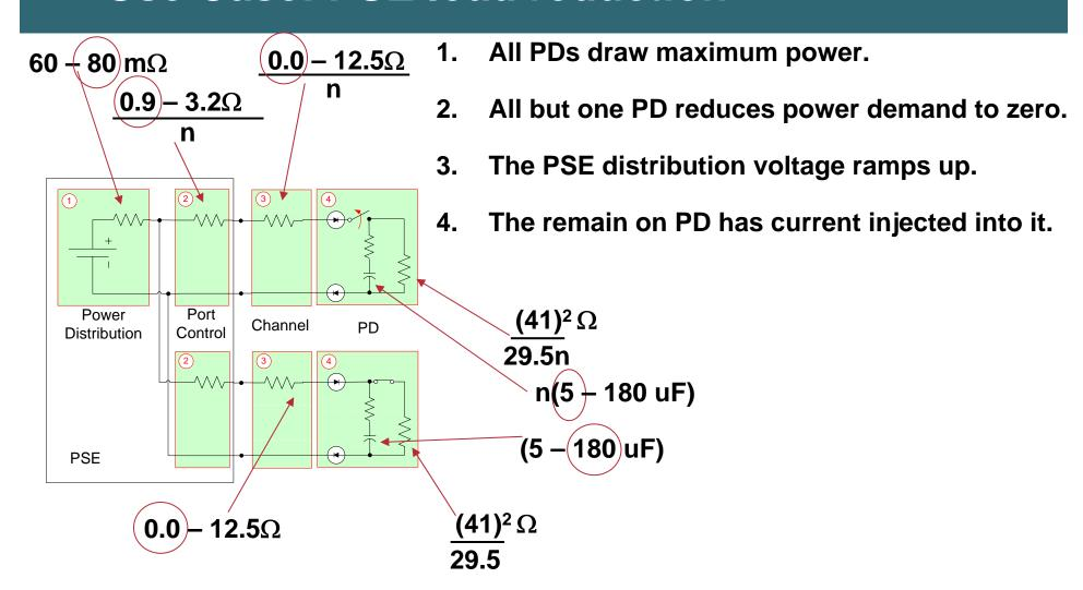
A PSE providing 50 V at 720 mA results in a PD voltage of 41 V (29.5 W).
