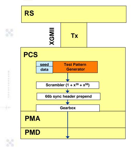
The test patterns are generated by utilizing the regular scrambler and framing mechanisms of 10G:
