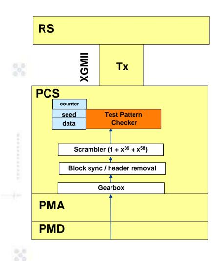
The test pattern data is received by the <u>Checker</u> function via the regular synchronization, framing, and scrambler mechanisms of Serial 10G:
