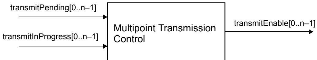
Figure 93-5—Multipoint Transmission Control Service Interfaces
